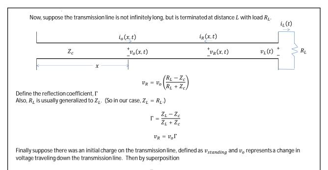
$v_L = v_{standing} + v_o + v_o \Gamma = v_{standing} + v_{incident} + v_{reflected}$
